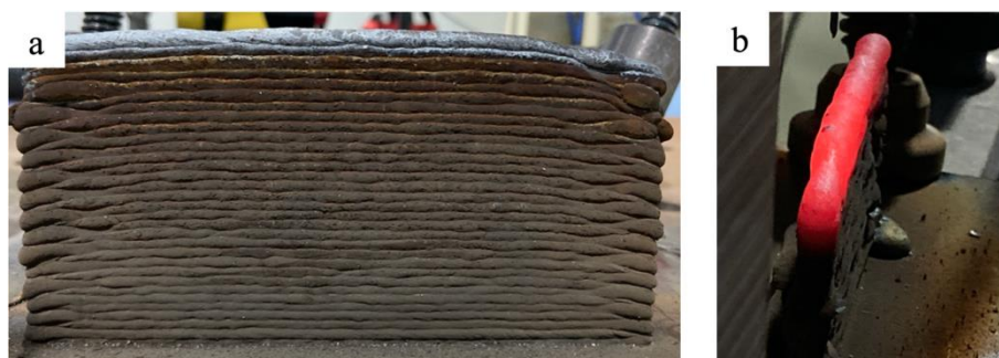
Figure 2 - Wire arc additive manufactured steel 9CrMoV-N samples (a – produced without a magnetic field, b – in a magnetic field (side view))
